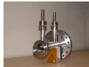
Dark current of 90keV is deflected in front of a **circular collimator** by **700 V DC**, this voltage droops to zero to 2 ns
